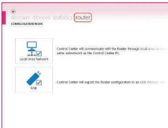
The C6 Router can be configured via two different communication paths:
