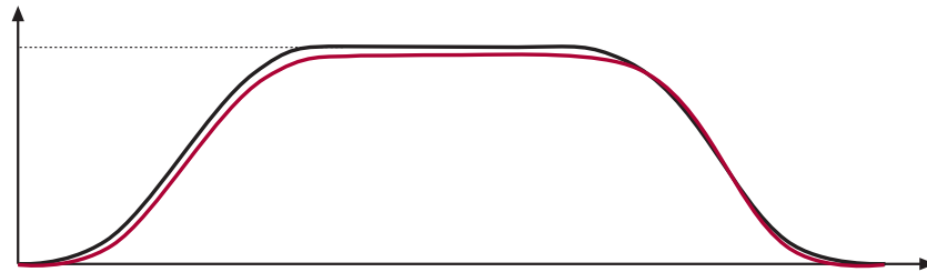
Integral Gain Too Low (100) - Speed Lags Command
